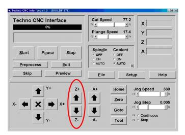
D. In the Interface, switch from **Continuous** to **Step** (just click on the **Step** radio button or pressing F8 on your keyboard, see picture).
