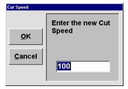
If you would rather not use the scroll bar to adjust the Cut Speed, you can double click the area above the Cut Speed Scroll bar and a shortcut menu (shown at left) will appear.
