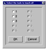
At this point you must click each tool # you want to calibrate the tool length offsets. Once selected, press OK and the machine starts to pick up and touch-off the tools. Again, this is done assuming you have the toolpad in position for the touch-off process.
