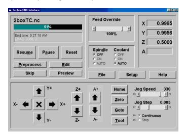
**Note:** When the file stops for the tool change, if the Z-axis is too low for easy-access, jog the Z-axis up and/or over to perform the tool change.
