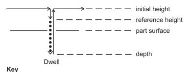
drill motion at plunge speed rapid motion at rapid speed
