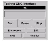
If any section of the Main Menu could be called the **CONTROL CENTER**, this portion would; simply because from here you can control the operation of the file: Start, Pause and Stop a program run, Edit code, view the file's toolpath and progress, etc. Next to the buttons below, we will explain and show the relevance of each of these **FILE EXECUTION CONTROLS**, including their respective windows.
