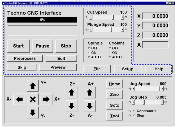
In any File Execution, the first step is to retrieve a file. The **File** button opens a window that allows you to search your PC to retrieve and open a file.
