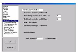
The **ADVANCED** tab represents the Factory Default values set for Speed rates, Acceleration rates, etc. The values represent maximum limits for each function. As the tab implies, these settings are not to be changed by the novice user.
