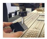
D. Manually lift the touchpad to the tool and then gently touch the pad to the tool (see picture above).
