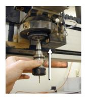
**Note:** Prepare to load tool holder 1 and close the chuck around it. Place the top of the tool holder cone all the way up into the spindle chuck. When the chuck closes, it will grasp the tool holder and lift it into the chuck a fraction of an inch. Allow for this lift.
