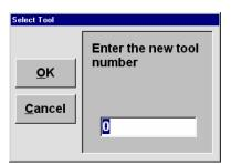
Press **THE IDENTIFY TOOL IN CHUCK** button when you need to identify the tool in the chuck. For instance, if after a software crash, the Interface does not remember what number tool is in the chuck, the interface, however, does remember the tool stand locations. So, if you input the tool number into the input box (shown at right) you will be able to return the tool to the proper tool stand.
