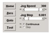
Set or change the **JOG SPEED** rate and **JOG STEP** size in any one of four ways. One, move the scroll bar. Two, use the arrows at either end of the scroll bar. Three, change the value by pressing the keyboard shortcuts, F5 through F8. Four, double click the area above the scroll bars and a shortcut window will appear. Simply, enter the desired vale in the input box and press OK.
