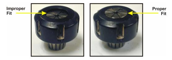
C. Press down on top of the collet nut to snap the two together for proper fit.
