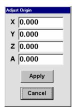
A shortcut window to manipulate the axes position will pop up when you double-click in the Position Display area. The purpose of this window (shown at left) is to be able to tweak the position counters while the program is in Pausemode. After you make the changes you want, click the Apply button and the changes will be made when after the window closes.
