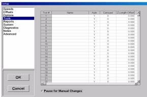
Location and Length Offset columns in the scrollable area get programmed automatically when you teach the Tool Stand Locations and Tool Lengths, respectively.
