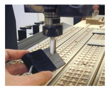
D. Manually lift the touchpad to the tool bit and then gently touch the pad to the tool.
