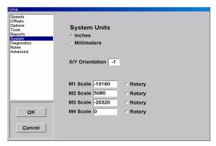
The **SYSTEM** tab refers to options for: units of measurement, machine orientation and motor scale factors. The X/Y Orientation is either +1 or -1. You can choose which one you want by clicking either button. Each button has a pictorial representing the positive directions of the X and Y-axes, from the reference point of you standing in front and facing the machine. The typical factory setting is set at -1.
