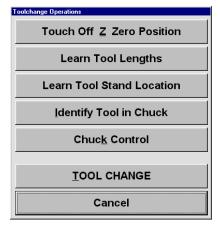
The **TOOLCHANGE OPERATION** window appears when you press Tool. This window will allow you to perform all the functions on the buttons contained within the window. The buttons and windows below show and explain these functions. Note: If you have not homed the machine before pressing the Tool button, this warning window (shown here) will appear.
