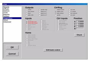
The **DIAGNOSTIC** tab is as a self-evaluation sheet for your machine and software, used in trouble shooting applications. If, for instance, you call for Tech Support, the Help Desk will more than likely direct you to the Diagnostic tab.
