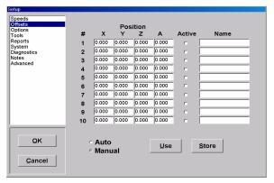
The 'offset' in **OFFSETS** tab refers to the work-piece or work-area offsets. Note that there is only one Active box checked; this is because you can only activate one set of offsets at a time. You can have several offset values inputted into the many rows available, but only one row can be active.
