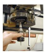
**Note:** When the chuck closes, it will grasp the tool holder and lift it into the chuck a fraction of an inch. Allow for this lift.
