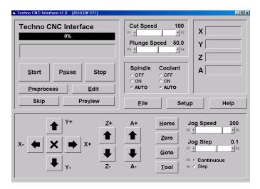
**Note:** This tutorial is written assuming your **X/Y Machine Orientation** is set to the Interface default setting of -1 If this has somehow been altered, go into **SETUP/SYSTEM** and make sure the X/Y Orientation is set to -1.
