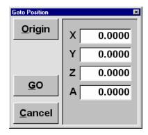
The **GOTO** button window allows you to move any axis to a specified location or move all of them to the machine Origin by pressing Origin.
