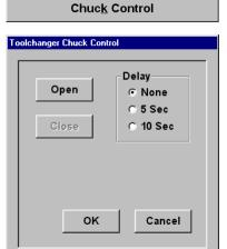
Press the **CHUCK CONTROL** button when you want to set the amount of time-delay before the chuck opens and releases the tool. Your options are None, 5 seconds and 10 seconds. The purpose here is to give you enough time to move from wherever your computer controls are to the spindle in order to catch the tool being released from the chuck.
