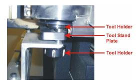
Warning: DO NOT go more than 3 clicks down on the Tool stand Plate (using a 0.01 Jog Step).
