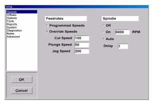
The **SPEEDS** tab allows you to adjust the Spindle's Speeds and feedrates. You have the option of using the CAD/CAM programmed speeds from your file or overriding the set federates and entering in new values in the Techno Interface. To choose the programmed speeds click on the Programmed Speeds radio button. This will grey-out the Cut, Plunge and Jog speeds. To ignore the programmed speeds and set them
