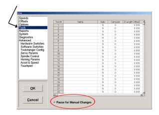
C. Select the Pause for Manual Changes function at the bottom of the Setup/Tools Window (see picture above). This function is activated when a check is in the box.
