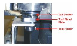
**Note:** From this position we begin the finishing touches for setting the tool stand location. We are going to do the following:
