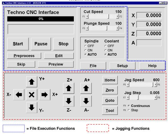
The Techno CNC Interface Main Menu is extremely user-friendly. There are two primary functions through which all the controls are used: **JOGGING** and **FILE EXECUTION**.
