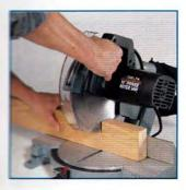
**Cressurs a nominal 2 x 6 or 4 x 4 at 90°.** Miters a 2 x 4 flat or on a single pass, at 45°.
