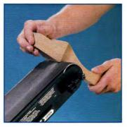
End of belt can be used for convenient contour sanding. Note that the belt operates at any angle between 0° and 90°.
