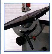
**Rack and pinion table tilt adjustment** for accurately setting table at any angle from 3° left to 45° right.
