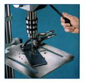
Twelve spindle speeds ranging from 250 to 3000 rpm for optimum drilling performance in a variety of materials.
