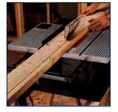
Integral outfeed work support handles large panels and long stock; slides in, out of the way, when not in use.
