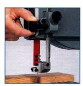
**Rack and pinion** Micro-Set® blade guide and guard system for precise height adjustment.
