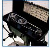
**Pivoting motor mount** to simplify speed changes and maintain correct belt tension
