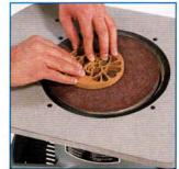
With the fence removed, you can take full advantage of this sander's large 9" diameter sanding pad and wide 22" x 16" table surface.
