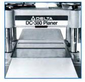
**Cutterhead assembly** features a patented adjustment system that acurately raises and lowers cutterhead on four precision-ground columns.
