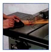
**Miter gage** has positive stops at 45° and 90° for accurate angle cutting. Compound angles can be achieved by tilting blade.
