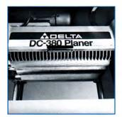
**Spiral serrated steel infeed roller** and polyurethane outfeed roller keep stock moving smoothly and efficiently.
