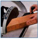
The Delta 12" Disc Sander features a 3/8" x 3/4" miter gage slot machined into the table for projects that require sanding an angle or stright edge.
