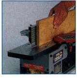
**Center-mounted fence** gives needed support throughout the cut for accurate edge jointing.
