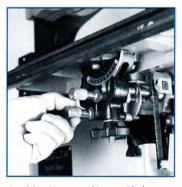
Precision Upper and Lower Blade Guides. Lower blade guides have safe, accurate, micrometer adjustment. Lower guides angled to support blade to within 3/4" of table work surface---assures accurate cutting.
