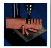
**Other useful operations** you can do using accessories include plug cutting and sanding.
