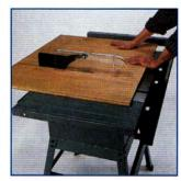
Full 221/4" x 38 1/6" table with extension wings and T-slot grooves provides ample work support for ripping large panels.
