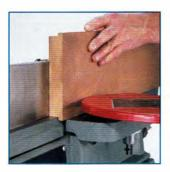
**Built-in rabbeting support ledge** allows you to make rabbet cuts with ease. Note that when the fence is moved forward it acts as a rear cutterhead guard.
