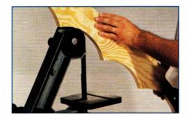
Belt cover is removable for access to the idler wheel when performing contour sanding operations.
