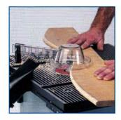
**Fence is removable** for freehand routing and shaping; an accessory insert accepts template guides for pattern routing.
