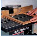
For increased flexibility, an accessory ½" arbor spindle is available for mounting ½" bore 3-lip shaper cutters.
