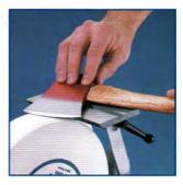
**Wet wheel** sharpens hardened cutting tools without damaging temper.
