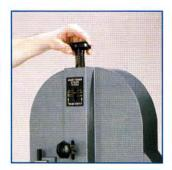
**Blade tensioning device** with handy scale and control knob to facilitate adjustment and setting for different width blades.
