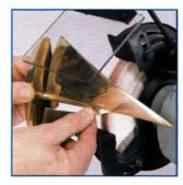
**Buff and polish** virtually any material using an accessory buffing wheel.
