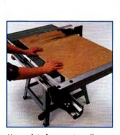
**Heavy-duty fence system** offers 30" capacity to the right blade for large ripping jobs.
