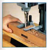
Fully adjustable fence/holddown assembly to accommodate various size work. Holddown prevents workpiece from lifting as chisel is withdrawn.
