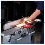
**Center-mounted fence** tilts 45° in and out. Acts as a rear cutterhead guard when fence is moved forward.
