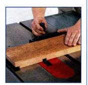
**Dado cuts** can be made in any width up to <sup>13</sup>/16" by mounting accessory dado and table insert
