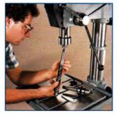
Tapered bits can be fitted directly into the spindle or mounted using the 3-jaw chuck with the spindle adapter included with the unit.
