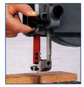
Rack and pinion upper blade guide adjustment offers precise movement for properly positioning blade guide above the workpiece.
