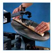
**Table tilts** for bevel cutting. Positive stop facilitates resetting to bevel position.
