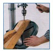
Large, precision-ground production table, with coolant trough and diagonal T-slot grooves, rotates and tills 90° left and right for angle drilling operations.
