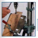
Titing table for angular drilling in side ledges and parallel slots for fast clamping of work.
