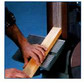
Cast aluminum table, with miter gage slot, may be used on either the belt or disc unit; tilts 45° for bevel sanding.
