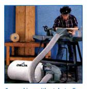
For machines without dust collection capability, the Delta Portable Dust Collector features a wide dust hood that can be positioned near the work area to help minimize the amount of dust build-up during woodworking operations.
