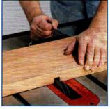
Cut dados at any width up to <sup>13</sup>/16" simply by mounting accessory dado and table insert.
