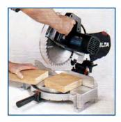
Crosscuts a nominal 2 x 6 or 4 x 4 at 90°. Miters a 2 x 4 flat or on edge at 45° R&L.
