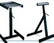
No. 50-298 Roller Stand ■ With 1.9" dia. x 12" ball bearing supported roller and dual widely-spaced base structure for stability. Adjustable in height from 25" to 42½". Folds flat for storage. Adequately
