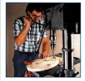
The production sized table tilts up to 45° left and right. Integral slots for clamping the workpiece.
