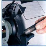
When equipped with a wire wheel, you can remove rust and scale from metals.
