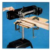
**Tilting head** permi**ts** horizontal drilling or boring operations in extra-long stock
