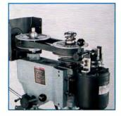
Variable speed drive system includes a jack shaft for providing full torque at any speed. High and low speed ranges offer infinitely variable speeds from 150 to 3200 rpm.
