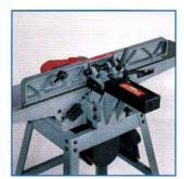
Center-mounted 4½" x 29½" fence for maximum work support throughout. Fence tilts for beveling and chamfering operations; features adjustable positive stops at 90° and 45° positions. Functions as a rear cutterhead guard on narrow cuts.
