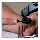
Quickset IP Blade Chuck and instantacting blade tension-release lever makes fast work of blade threading for internal cutting.
