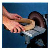
**Large 9" diameter abrasive disc** is perfect for sanding large curves or rounding out sharp corners.
