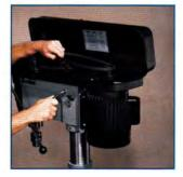
A quick release motor mount loosens belt tension for fast and easy speed changing.
