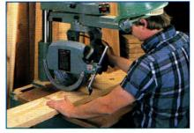
**Powerful Motor with Mechanical Brake.** 2 HP motor develops up to 4 HP peak under heavy workloads. Mechanical brake stops blade automatically in seconds.
