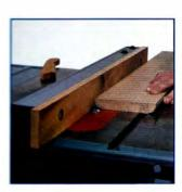
Moulding operations can be parformed using the accessory cutternead and table insert
