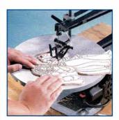
**Easily makes smooth internal cuts** on even the most intricate fretwork.
