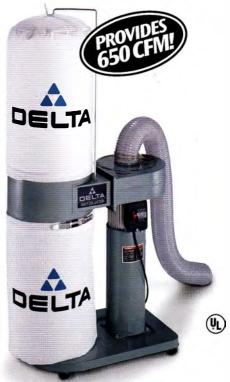
Model 50-840 1 HP Single-Stage Dust Collector ■ Includes basic machine with 1 HP motor and blower, 2 collection bags, support drum, 4" diameter hose, base with four swivel caster assemblies, cord and plug, and instruction manual.
