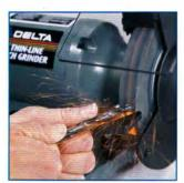
**Sharpen drill bits**, lathe chisels and other workshop cutting tools.
