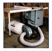
Remove the dust hood, and the vacuum hose of the Portable Dust Collector can be fitted with any variety of connectors that accept a 4' diameter hose. We show it here with a the Delta No. 50-236 connector.
