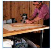
The Portable Dust Collector is compact enough to fit underneath your workbench for clamping dust hood to the top of the work table for routing or sanding operations.
