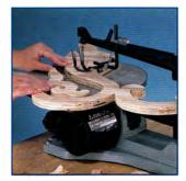
Offers 16" arm-to-blade capacity for large-capacity curve cutting.
