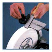
**Single angle jig** facilitates sharpening of double angle cutting tools.
