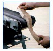
Adjustable belt unit operates vertically, horizontally or at any angle in-between for operator convenience. Upper belt guard can be removed for contour finishing on idler drum.
