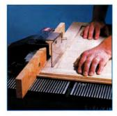
Accepts all 1/2" and 1/4" shank router bits for cutting mouldings, decorative edges and common wood joints.
