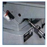
**Quick-index infeed table positioning lever** for fast, accurate set-up. New depth-of-cut scale has highly visible pointer and markings, and adjusts easily with one simple lever.
