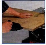
**T-slot grooves** hold miter gage securely beyond front of table, preventing it from falling during wide cut-off operations.
