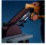
**Adjustable belt unit** operates vertically, horizontally or at any angle in-between. Belt guard removes easily for contour sanding.
