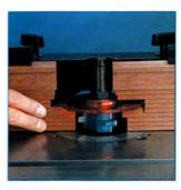
Patented fence conforms to cutter shape for improved chip removal and dust collection; greater operator protection.
