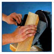
Table tilts 45° for bevel sanding; compound angles can be achieved using standard equipment miter gage.
