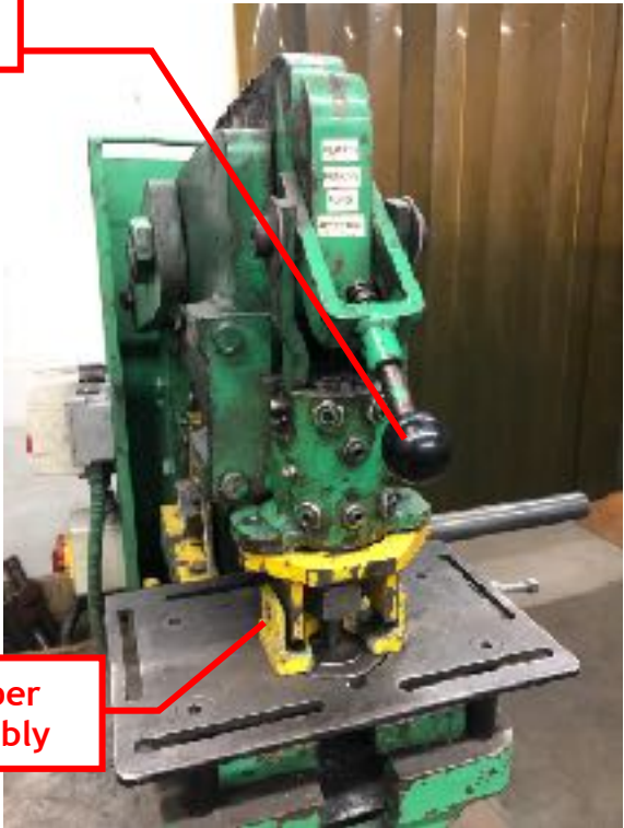
Punch Installed , with Punch Release handled lowered to check die alignment.
