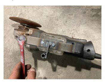
Clamping force is provided by the wingnut holding the cleat sleeves to the  $3/8-16 \times 6$ " bolt on the base, when the grinder is mounted to the gantry.
