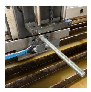
Use the middle set of holes in the base plate as shown. Two sets were drilled wrong. Tighten the nuts with lock washers to hold the base tightly to the gantry.
