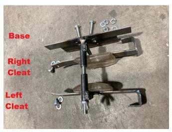
The fixture has 3 major parts, a base and two cleats. Also included are 2 M8-1.5 x 30 mm bolts, 2 M8-1.5 x 12 mm bolts, 2 M8-1.5 nuts, washers, lockwashers, and one 3/8-16 wing nut.
