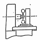
Place a cylindrical square gauge on the table top to get in touch with the dial indicator pointer attached to the spindle head. Read the value at the top, then swing the spindle 180 degree to the bottom position and read the value again.
