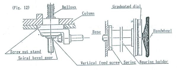
3. By the spiral bevel gears and ball bearings of this parts, the light driving of feed without and play and noise is completely assured. Also, the below around the male screw doubly protects the feed from the dust, and there is scarcely any damage due to the dust.
