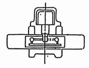
Place a square surface plate on the table parallel to the longitudinal table drive.
