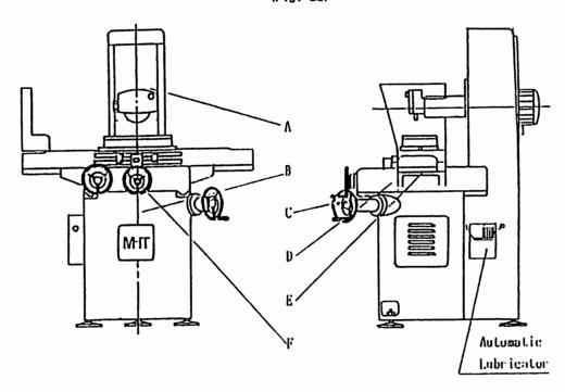
A,B,C and D are automatically lubricated by Model-MLZ Automatic Lubricator located right-hand side back of machine base.
