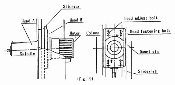
Adjustment of head-slideway clearance
