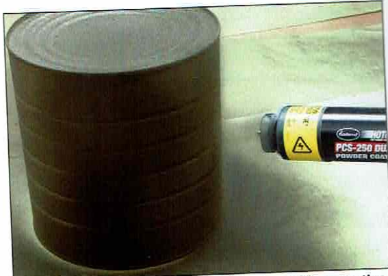
Powder is "wrapped" around all sides by static attraction
